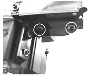
View of two motor adjusting bolts under motor bracket.
